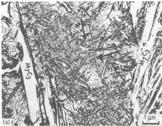
Figure 3 Optical microstructure of irons after heat treating, note numerous secondary carbides in dominantly martensitic dendrites. Etchant: Kallings's Reagent for (a) Alloy A4, and Vilella's Reagent for (b) Alloy B4 and (c) Alloy C4.
